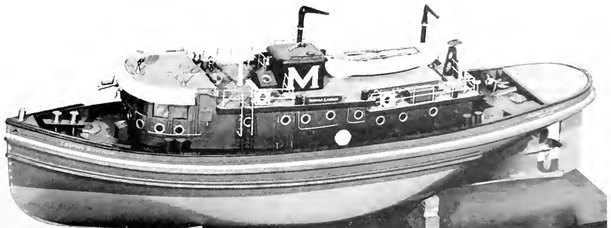
RIGGED MODEL (USNM 312088) OF THE MODERN STEEL, DIESEL HARBOR TUGBOAT Thomas E. Moran , 1938. Tugs of this type have displaced the older wooden and steel tugs in the large American ports. (Smithsonian photo 44997-j.)
